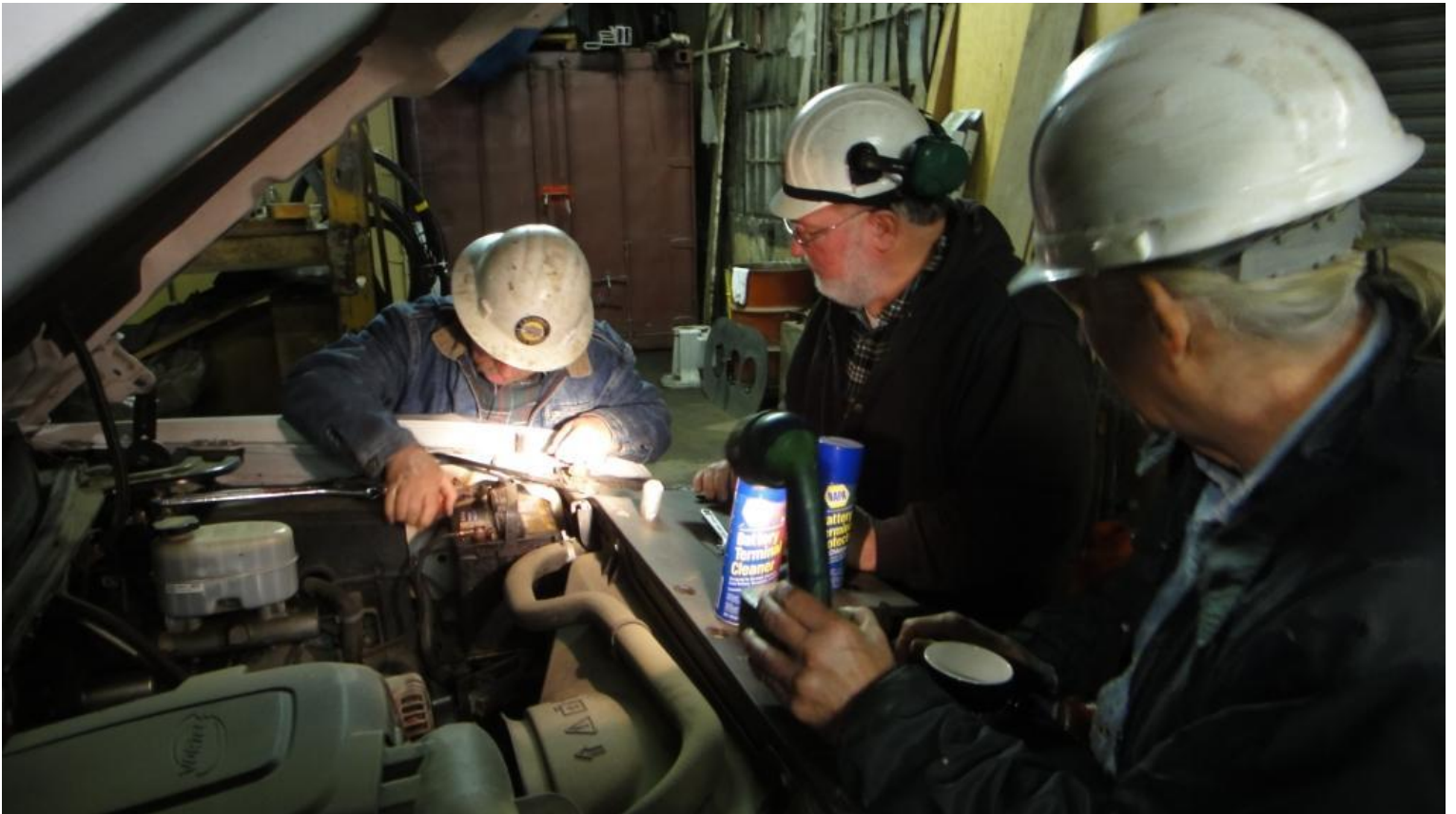
Mike H. and Frank replace the battery terminals on the trusty Chevy Truck. Fred provides the light
